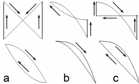
**Figure 3:** Hysteresis loops for the elastic modulus  $\partial \sigma_H / \partial s$  (upper row) and for stress-strain correction  $\sigma_H(s)$  (lower row) in the case of friction-type hysteresis (a) and for adhesion-type hysteresis: (b) – parameter  $\rho=0$  (elementary triangle), and (c) parameter  $\rho=1/2$  (elementary trapezoid).
