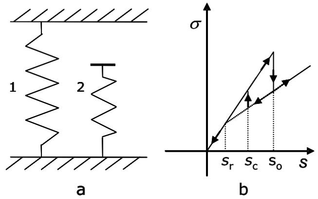
**Figure 2:** (a) Schematically shown adhesion-type hysteretic element in which part 2 may lost and restore adhesion contact. Plot (b) represents for such an element its stress-strain loop of a trapezoidal form that reduces to triangular one in the ultimate case when characteristic strains  $s_c$  and  $s_r$  coincide, so that parameter  $\rho = (s_c - s_r)/(s_c - s_r) = 0$ .
